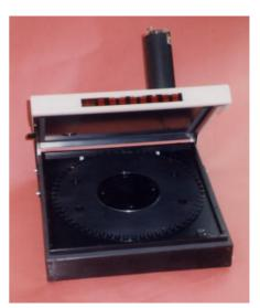
The 2200 automated OSL reader is the latest in the Daybreak TL/OSL family, providing the functions of a sample changer, irradiator, and preheater in a single package. Mechanically simple, like the Daybreak 801E multisample irradiator, the model 2200 has a single demountable 40 cm platter to hold 60 samples. The total
