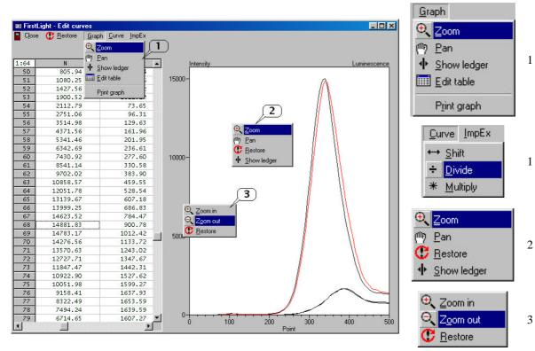
Below we see an example of a complex system of interacting windows, presenting measurement data and analysis results, during the growth curve fitting and computations of the paleodose. An action taken by the user in any of these windows is reflected in all the others. This is achieved by applying the messaging system – windows send and receive messages to and from each other to notify about changes in data made by the user or changes in results generated by the program.
