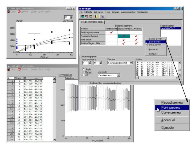
Results of computations are presented in several forms simultaneously. The 'Solution' sub-window in the main window (upper – right part above) contains numerical results of computations that may be easily transferred to an external file or directly to (through a Windows clipboard) any other spreadsheet or text editing program.
