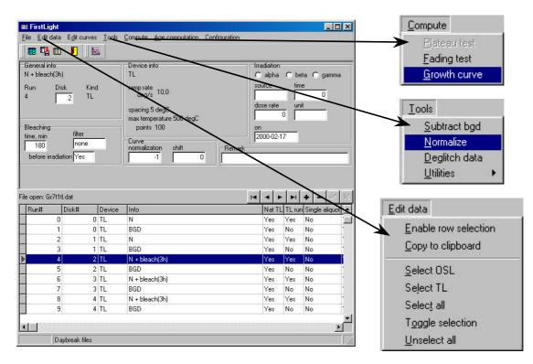
The top portion of the window displays the data from the selected curve in a readily intelligible form with fields derived from the data base. We store a very complete set of data as measurements are made, all defined by the script or batch program as it is executed. No post-processing is necessary as with other software.
